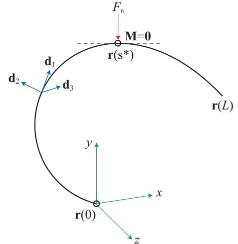
Figure 1: Coordinate systems for a whisker in point contact with an object at  $s = s^*$ . For frictionless contact the contact force  $F_n$  is normal to the whisker.
