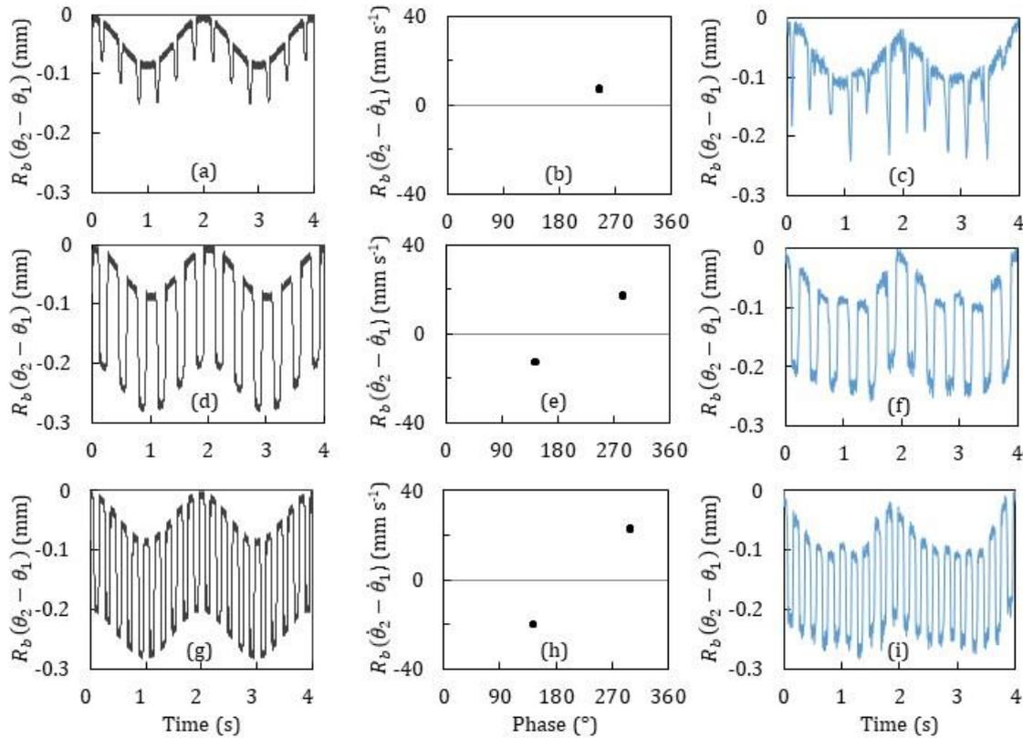
Figure 1: Impact response (numerical transmission error, Poincaré section, experimental transmission error) for several velocity fluctuation frequency and amplitude.
