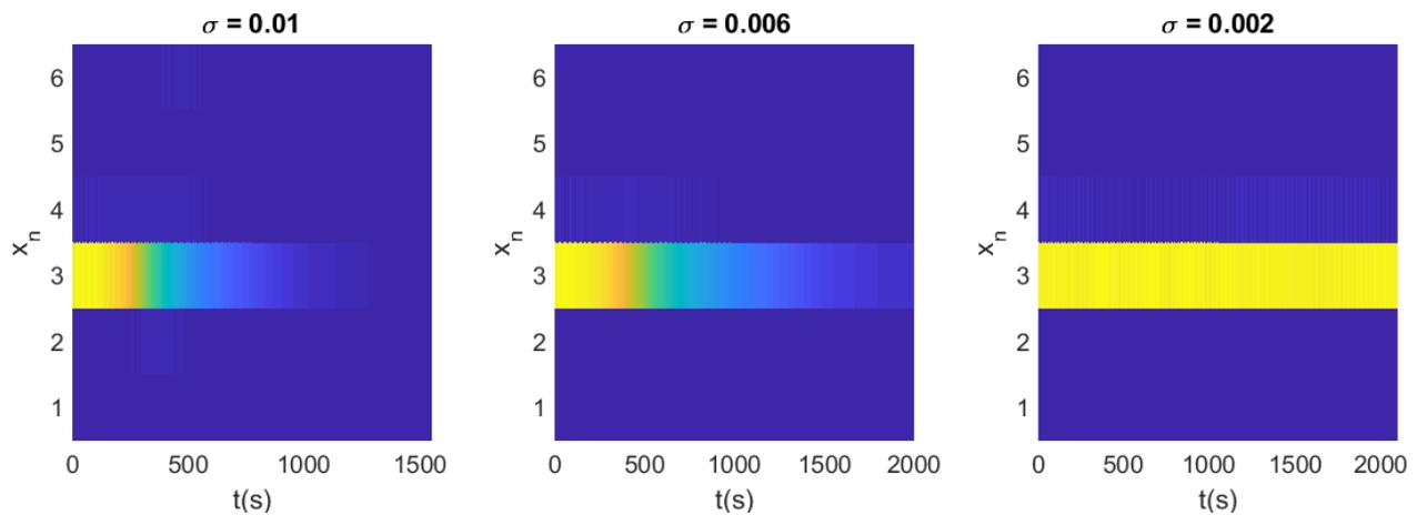
Figure 2: Energy distribution in a circular Duffing oscillator array averaged over 400 simulations. In all three cases, the energy is localized in the 3<sup>rd</sup> oscillator in the beginning. Addition of noise with intensity  $\sigma = 0.01$  and  $\sigma = 0.006$  can suppress the energy localization, and lead to a uniform energy distribution in the array. However, a lower noise intensity ( $\sigma = 0.002$ ) is found to be inadequate for pushing the system to the unison-amplitude mode.
