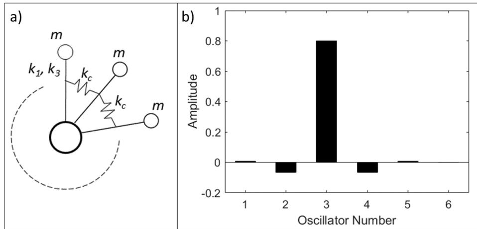
Figure 1: a) Coupled circular Duffing oscillator array with periodic boundary conditions. b) Amplitude profile of the localized mode: The energy is localized in the 3<sup>rd</sup> oscillator, and the amplitude profile is symmetric about the oscillator with the highest amplitude.
