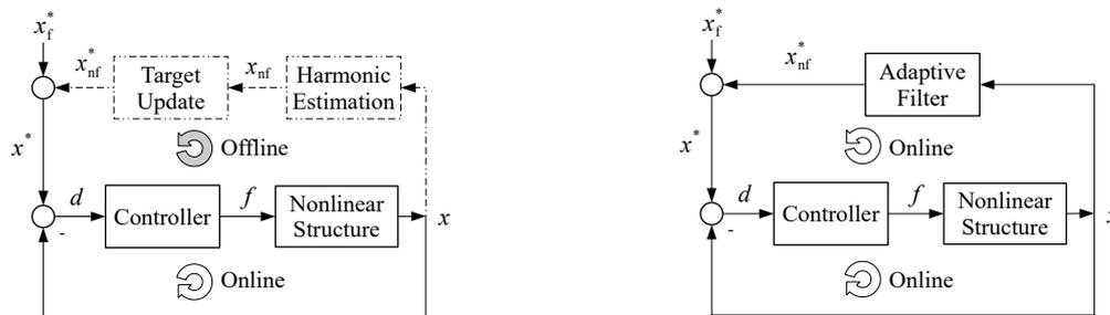
(a) Offline iterations on the non-fundamental target  $x_{nf}^*$ ; the dashed-dotted line is performed offline, i.e. at a much lower frequency (state of the art)
