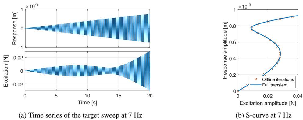
Figure 2: The relationship between excitation and response amplitudes (S-curve) can be obtained by sweeping the target amplitude
