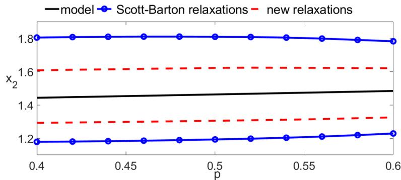
Figure 2: The final state  $x_2(t_f, p)$  vs.  $p$  (black-solid), along with corresponding Scott–Barton relaxations (blue-circled) and new relaxations (red-dashed), plotted as functions of  $p$  at  $t := t_f$ .
