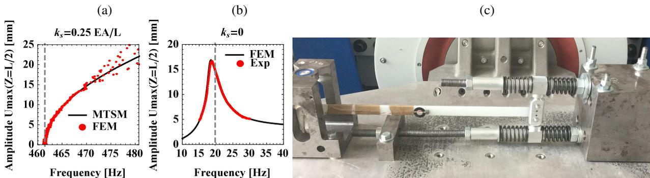
Figure 2: Free nonlinear oscillations (a), forced damped oscillations (b) and experimental setup - side view (c).
