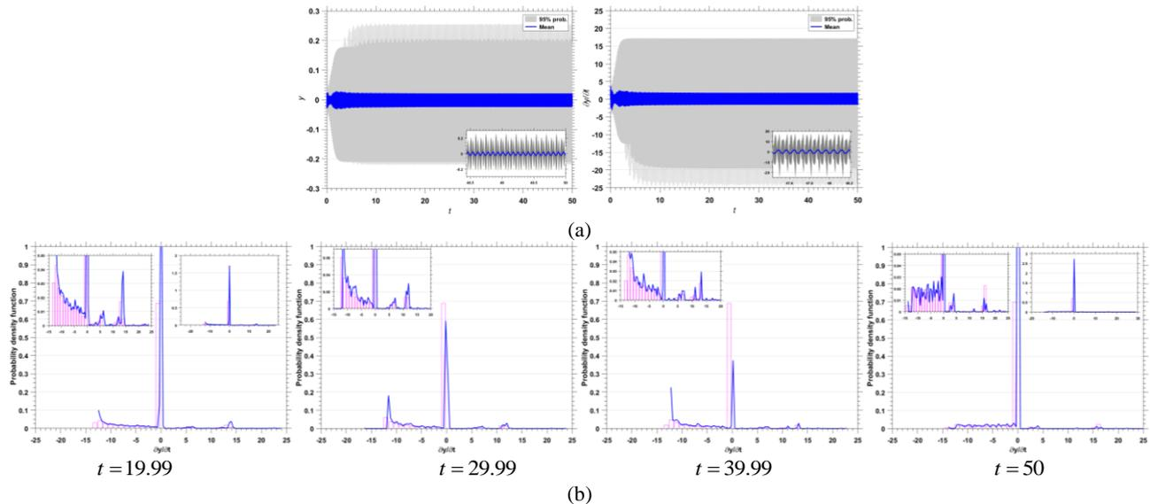
Figure 2:  $\Omega/2\omega_1 = 0.464$  (a) Illustration of the nominal value (Blue line) and the 95 % envelop (grey shadow) of the displacement (left) and the velocity (right) of the riser. The box in each figure is a magnified response of the riser. (b) Evolution of the normalized probability density function as a function of the rise velocity at different times. The box in each figure is a magnified distribution of the probability density function.
