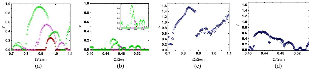
Figure 1: Multi-modal Frequency response curves around the first mode of vibrations for  $V = \sqrt{\sigma}$ ,  $c_d = 0.416$  at  $x=0.48$ . (a,b) Backward Sweep (  $\square$  )  $\gamma = 0.25$ , (  $\triangle$  )  $\gamma = 0.50$ , (  $\circ$  )  $\gamma = 0.75$ . The inset is magnified results for case (b). (c,d) (  $\diamond$  )  $\gamma = 1$ . Filled shapes denotes forward sweep.
