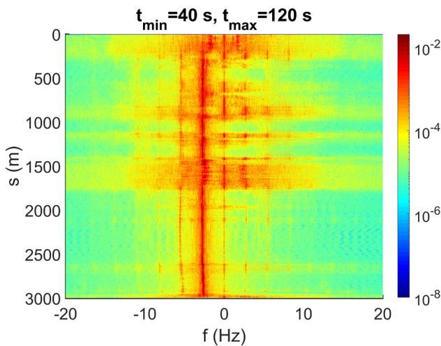
Fig. 3. Full spectrum analysis all along the drillstring.
