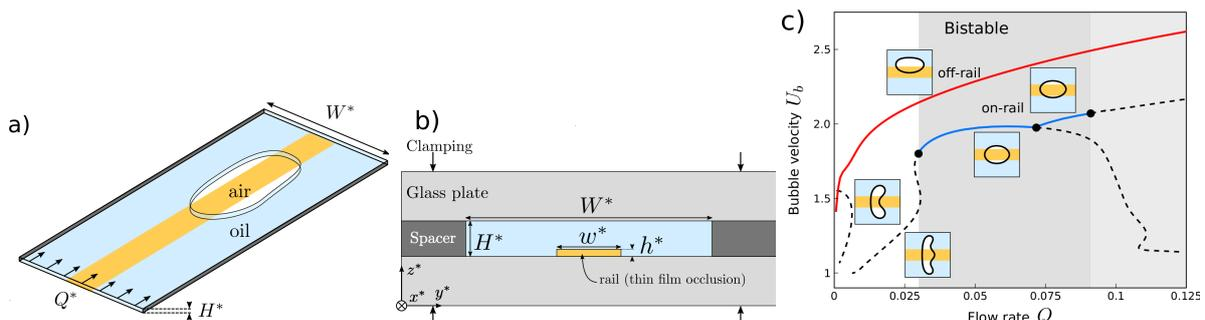
Figure 1: (a) Top-view of the experimental channel with an axially uniform, centred rail. (b) Cross-section of the channel. (c) Numerical bifurcation diagram depicting the steady modes of bubble propagation in terms of the bubble velocity as a function of the flow rate [5]. Stable and unstable modes are indicated by solid and dashed lines, respectively.
