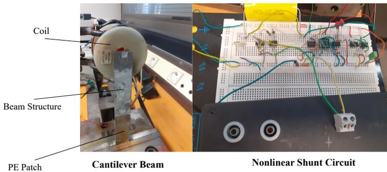
Figure 3: Experiment Setup
