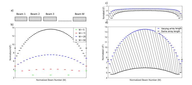
Figure 1: (a) Array of beams in non-viscous fluid (b) Absolute pressure for different array sizes (c) Real pressure and (d) Imaginary pressure for 50 beams array at  $\bar{g} = 0.1$  and Re = 0.1.
