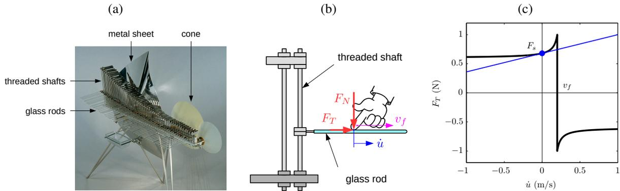
Figure 1: (a) Cristal Baschet (adapted from [1]). (b) Interaction between wet finger and resonator. (c) Friction curve and its linearization around static equilibrium in sliding situation.
