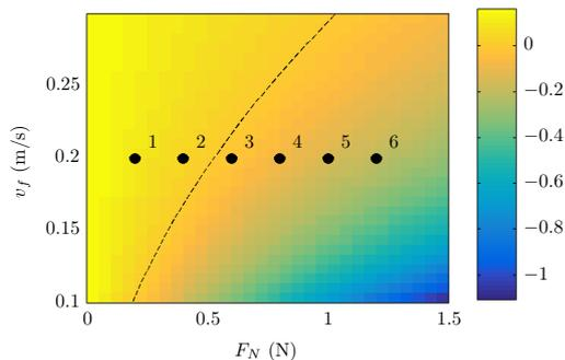
Figure 2: Smallest effective damping ratio  $\xi_{\text{eff}}$  as a function of the normal force  $F_N$  exerted by the finger and its velocity  $v_f$ . The dashed line indicates the limit between positive and negative values of the damping ratio, corresponding to stability or instability of the static equilibrium in sliding situation.
