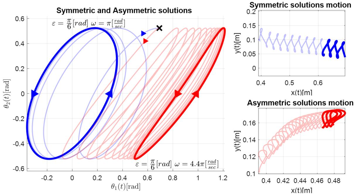
**Figure 2:** Transient simulations – Left: trajectories in joint-angles plane. Right: trajectories in x-y plane. **Blue:** symmetric solution, **Red:** asymmetric solution. Simulations with the same amplitude and initial condition and different frequencies result in significantly different solutions trajectories.
