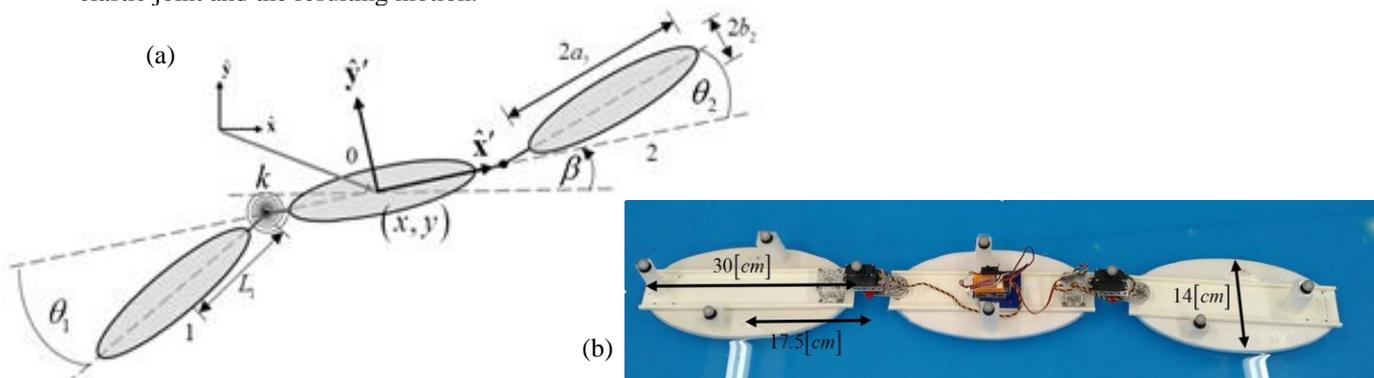
Figure 1: **(a)**. Swimmer model –  $(x, y)$  are the position of the body-fixed reference frame origin.  $\beta$  is the rotation angle of the body-fixed reference frame.  $a_i$  and  $b_i$  are the major and minor radii of the elliptical links.  $\theta_i$  are the relative angles between links. **(b)**. Our previous experimental robotic swimmer with two actuated joint angles [4]
