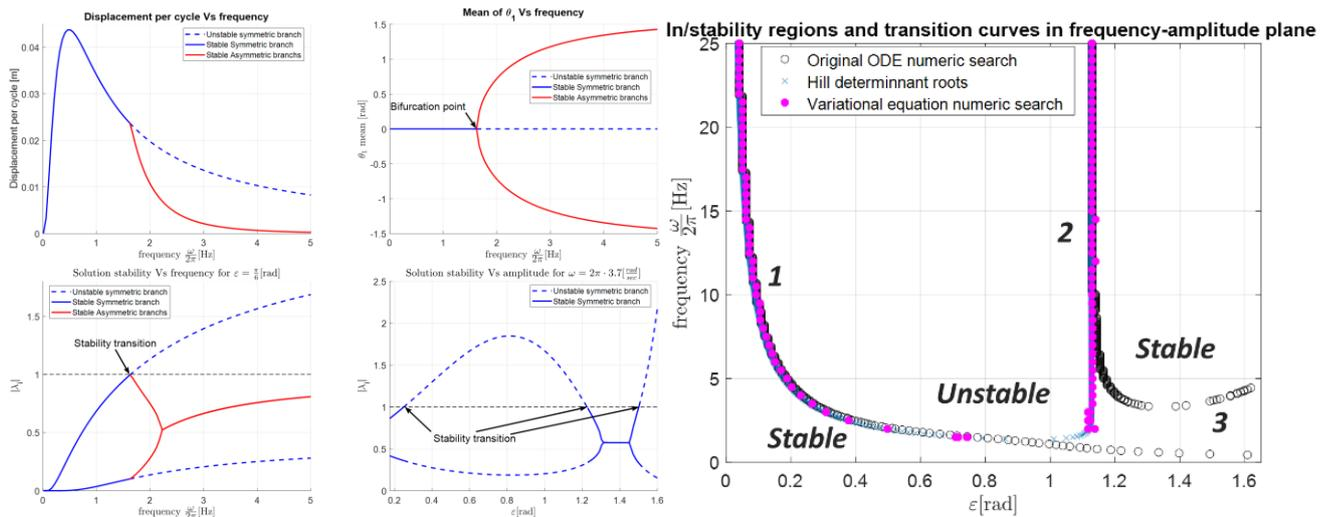
**Figure 3:** Steady state solution parameters in  $\omega$  and  $\varepsilon$  – Optimal frequency is found where the net displacement per cycle is maximized. A bifurcation point depending on input's amplitude and frequency occurs, where the symmetric solution loses stability and a pair of stable asymmetric solutions evolve. Stability transitions involve Floquet multipliers crossing  $|\lambda_i|=1$ .
