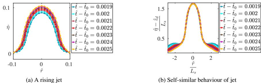
Figure 2: Panel (a), (b): Self similar behaviour of the jet at  $\epsilon = 2.0$  and cylinder radius  $R_0 = 2.936$  cm, where  $R_0$  is the radius of the cylinder. Here  $\hat{t}_0$  is the dimple formation time,  $\hat{\eta}$  is dimensional interface and  $\hat{r}$  is dimensional radial distance,  $\hat{z}_d$  is the height of the jet base (all variables with hat are dimensional)
