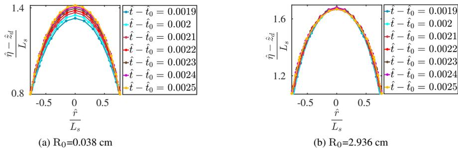
Figure 4: Panel (a), (b): Effect of container radius on the self similar evolution of jet
