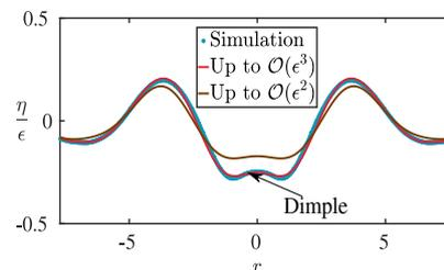
Figure 1: Comparison of the surface evolution of the interface at steepness  $\epsilon = 0.8$ . Numerical solution to the Euler's equation ( $\bullet$ ) using Basilisk [9],  $\mathcal{O}(\epsilon^3)$  ( $\text{---}$ ),  $\mathcal{O}(\epsilon^2)$  ( $\text{---}$ ). Third order theory captures the dimple very accurately. Here  $\eta$  is non dimensional interface and  $r$  is non-dimensional radial distance.
