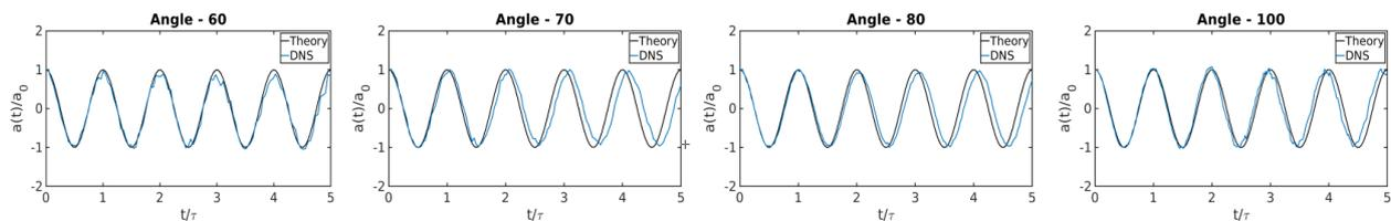
Figure 3: Oscillatory response obtained from numerical simulations in the bubble limit ( $\rho^O/\rho^I = 1000$ ) and comparison with linearised predictions [3]. A reasonably agreement is seen in all cases for comparison of linear theory with simulations.
