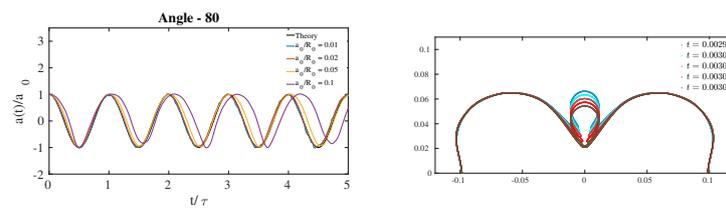
(a) Effect of changing perturbation amplitude (b) Droplet ejection during oscillation for  $a_0/R_0 = 0.3$
