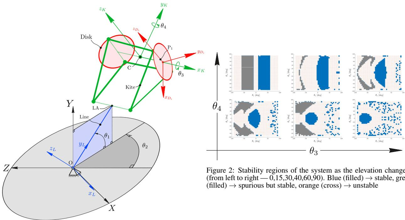
Figure 1: Coordinate systems for the two line kite
