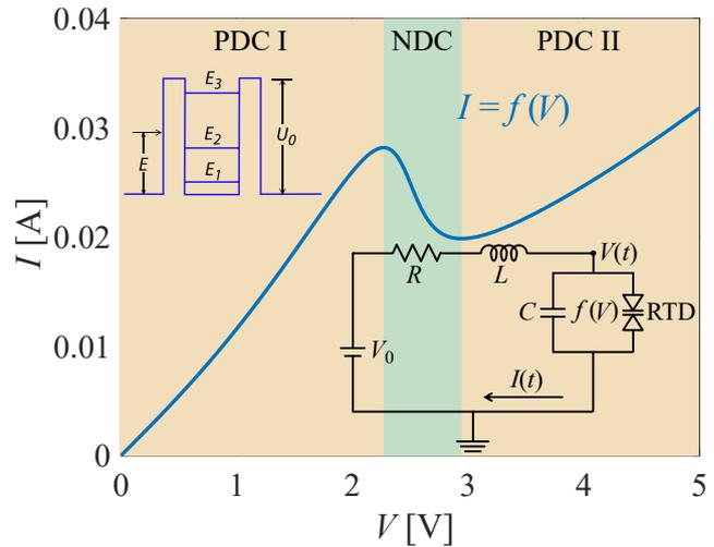
Figure 1: DBQW RTD connected to DC voltage.
