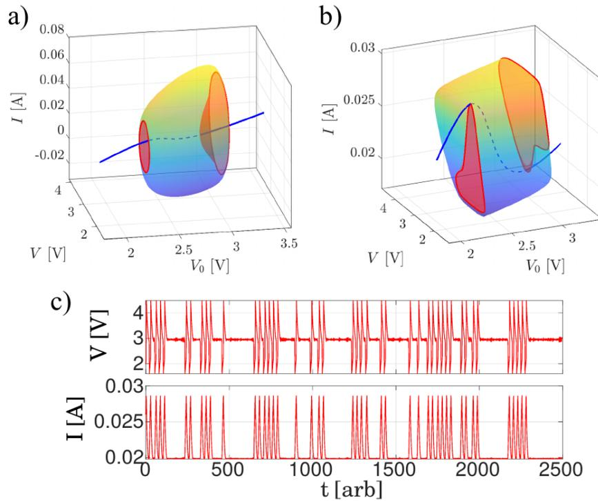
Figure 2: a,b) RTD response as a function of the bias voltage. Limit cycles are smooth (a) or stiff (b) depending on the stiffness coefficient. c) RTD response to external noise in the form of bursts of spikes.
