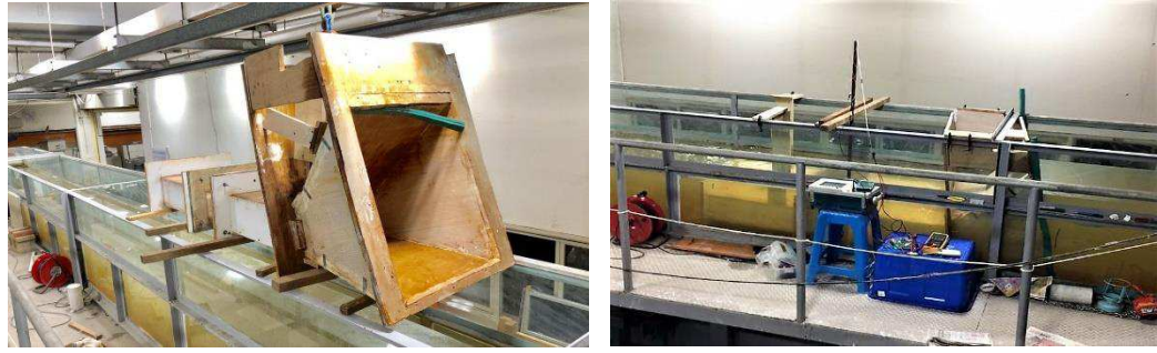
Figure 2. Flow field experimental equipment (a) Giant venturi tube, (b) Recirculating flume with giant venture
