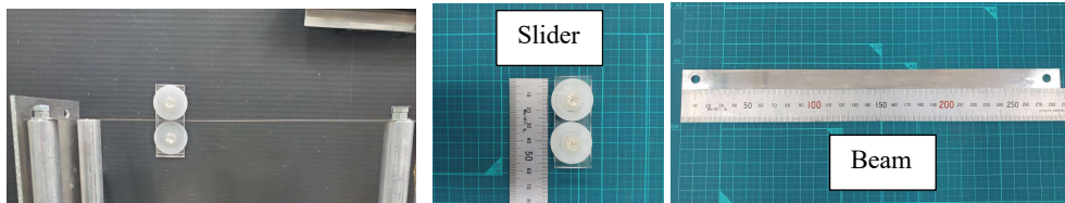
Figure 3: Picture of the experimental system of the beam-slider structure and its separated parts.
