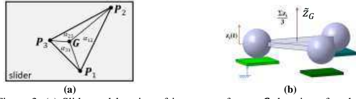
Figure 3: (a) Slider and location of its center of mass G , location of each contact point P_j , and area coordinates \alpha_{ij} ; (b) the equivalent sliding system.
